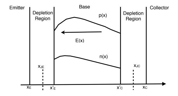
Since current density  $J_n$  is constant for dc and is independent of x, assuming negligible recombination in the base region (recombination in the depletion region is independently modelled by the two non-ideal of Gummel Poon Static Model, so it is assumed to be zero here),  $J_n$  is taken out of the integral. Then
