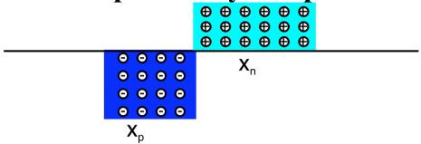
We have a charge separation and hence there is a capacitance associated with a pn junction
